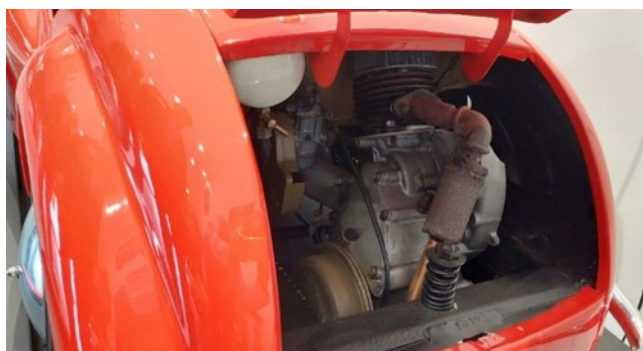
'The J40 engine from a 50cc Vespa scooter.
